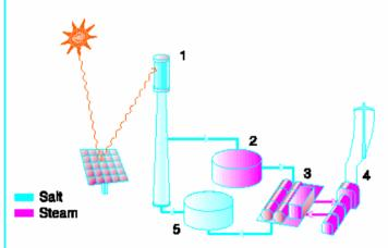
Schematic of electricity generation using moltensalt storage:
