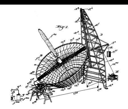
Patent drawing for Aubrey Eneas's second solar motor, 1899. To follow the sun's motion, the truncated cone mirror was moved along a track in tower scaffolding at right.
