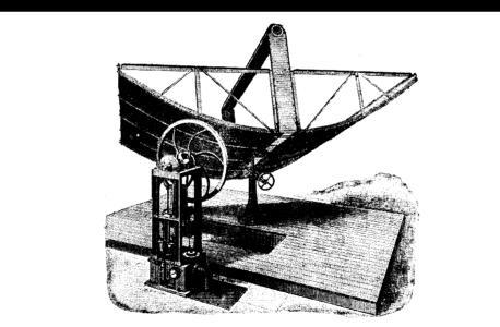
John Ericsson's solar motor, the first to use a "parabolic trough" collector (the curved shape that looks like a section of metal barrel). Frank Shuman later enlarged and adapted this design for his solar machine in Egypt.
