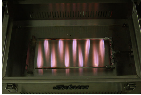
Figure 3.13: Hydrogen retrofit burner for the Solaire grill
